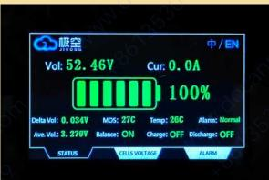
Click the switch button on the display screen and then click confirm to check if the battery starts normally.
